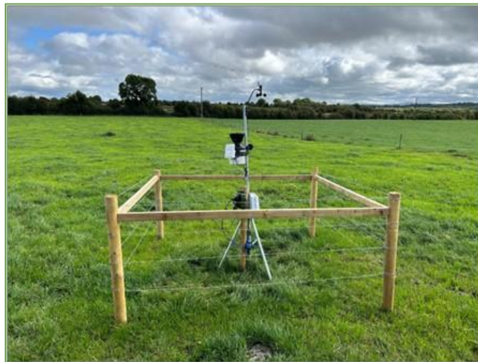
Plate 2.7 - Weather station erected at a suitably safe location within the proposed wind farm development site.
