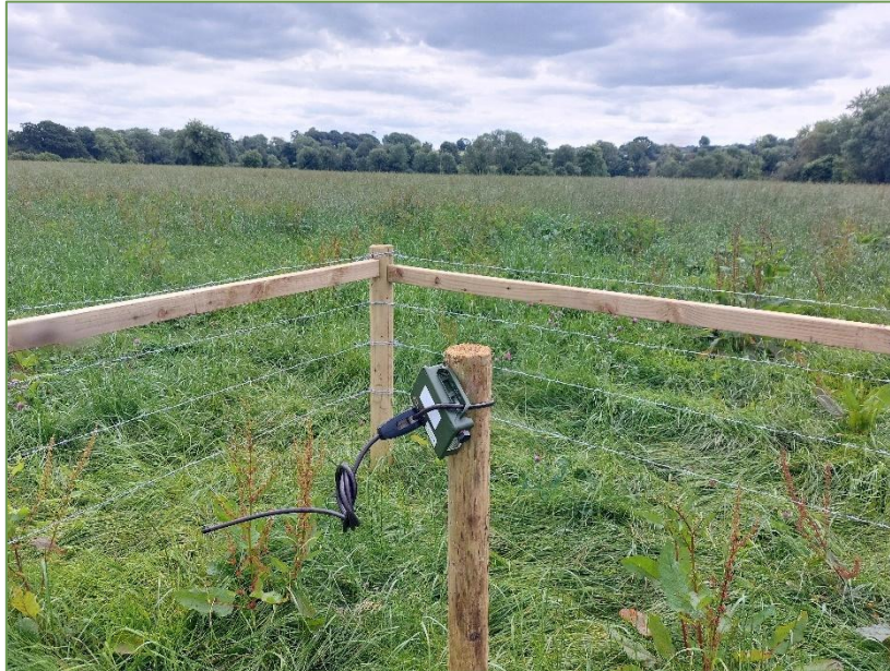
Plate 2.6 – Song Meter Mini Bat Ultrasonic full-spectrum detector deployed at a proposed Turbine location.
